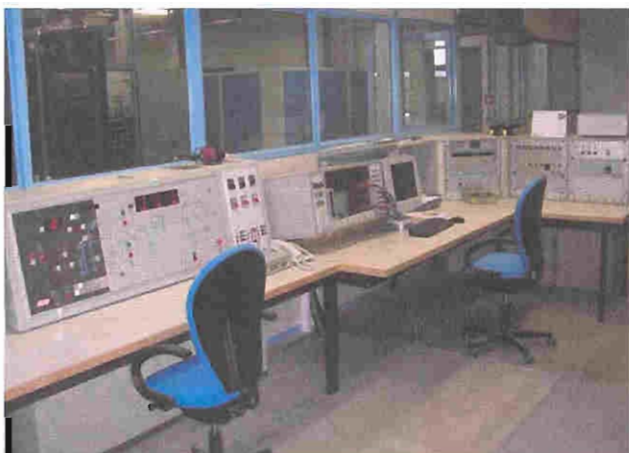
Control station for tests up to 15kA
