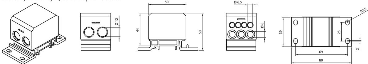
EDBM-2, EDBM-2/N, EDBM-2/PE - 50 mm<sup>2</sup>
