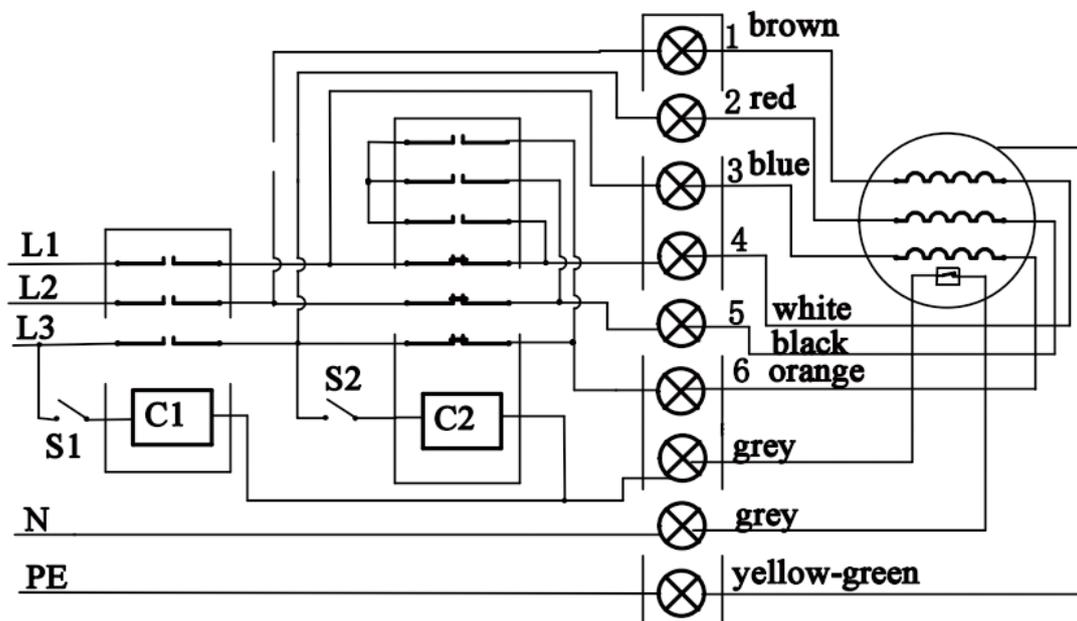
QF1 - run control air switch, QF1 switched on, the fan running. C1 - Y/Δ operation control contactor, S1 disconnect, Δ connection; S1 connected, Y connection.
