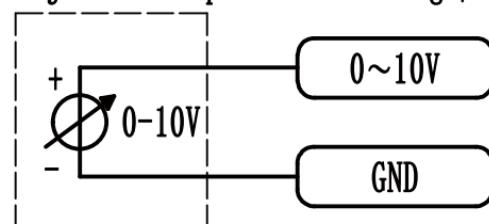
Adjustable speed via potentiometer
