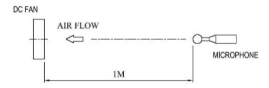
Noise Is Measured At Rated Voltage In Free Air In Acoustical Chamber With Larson Davis Type 824S Sound Level Meter
