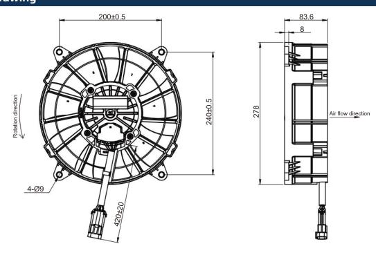
All dimensions in the above figures are in mm. Use M8 bolts to fix the fan, and the nominal maximum tightening torque is 5(+1/0)Nm. The definition of the nominal tightening torque applies to new, clean and lubrication-free bolts.
