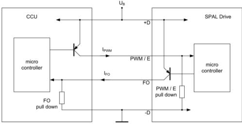
The circuit of the CCU and the circuit driven by the fan are connected through two unidirectional wire harnesses.
