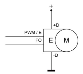
E represents the entire circuit part, and M represents the motor. Drive stands for the integration of motors and circuits.
