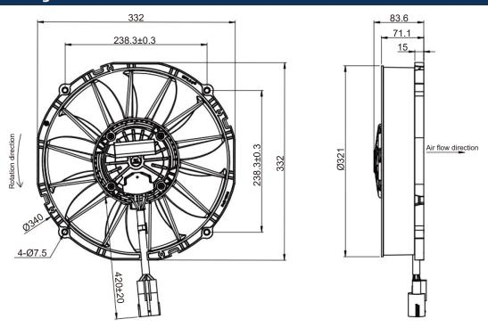
All dimensions in the above figures are in mm. Use M6 bolts to fix the fan, and the nominal maximum tightening torque is 3(+1/0)Nm. The definition of the nominal tightening torque applies to new, clean and lubrication-free bolts.
